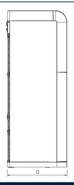
Dispensing Technical Data WxDxH (mm) weight **HYDRAZON 15** 350x416x1093 21 kg 280 mm **HYDRAZON 15 Fizz** 350x416x1093 25 kg 280 mm **HYDRAZON Hot 15** 350x416x1093 26 kg 280 mm **HYDRAZON Hot 15 Fizz** 350x416x1093 30 kg 280 mm
